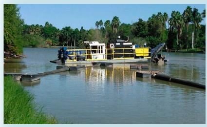
Floating dredger from IMS Dredges<sup>®</sup> is self-propelled and has a 9-foot cutterhead. Sediment is transported via floating pipe to an offsite dewatering system. **Credit:** Brownsville Public Utilities Board.
